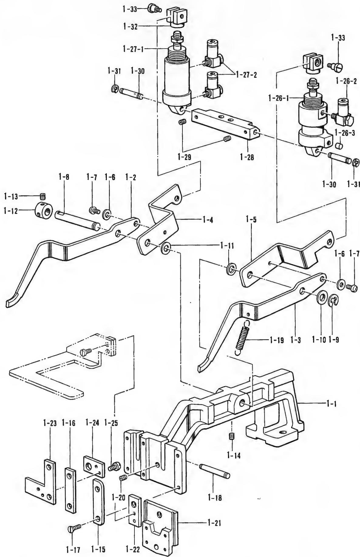
C. 送り関係/Feed mechanism/Transportvorrichtung/
