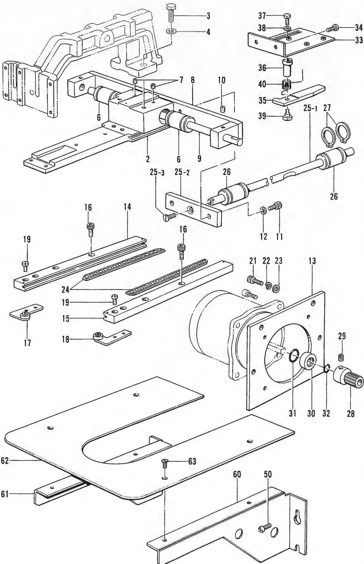
C. 送り関係/Feed mechanism/Transportvorrichtung/
