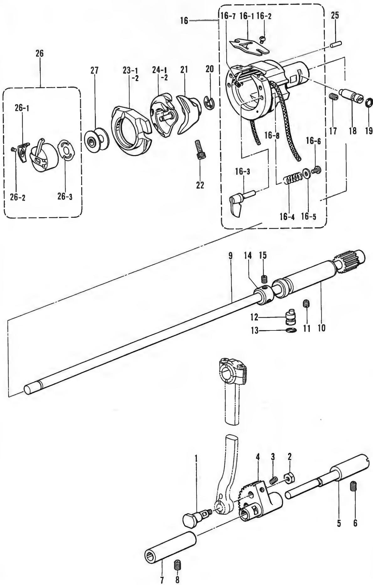
F. 下軸関係/Lower shaft mechanism/Untere Welle/
