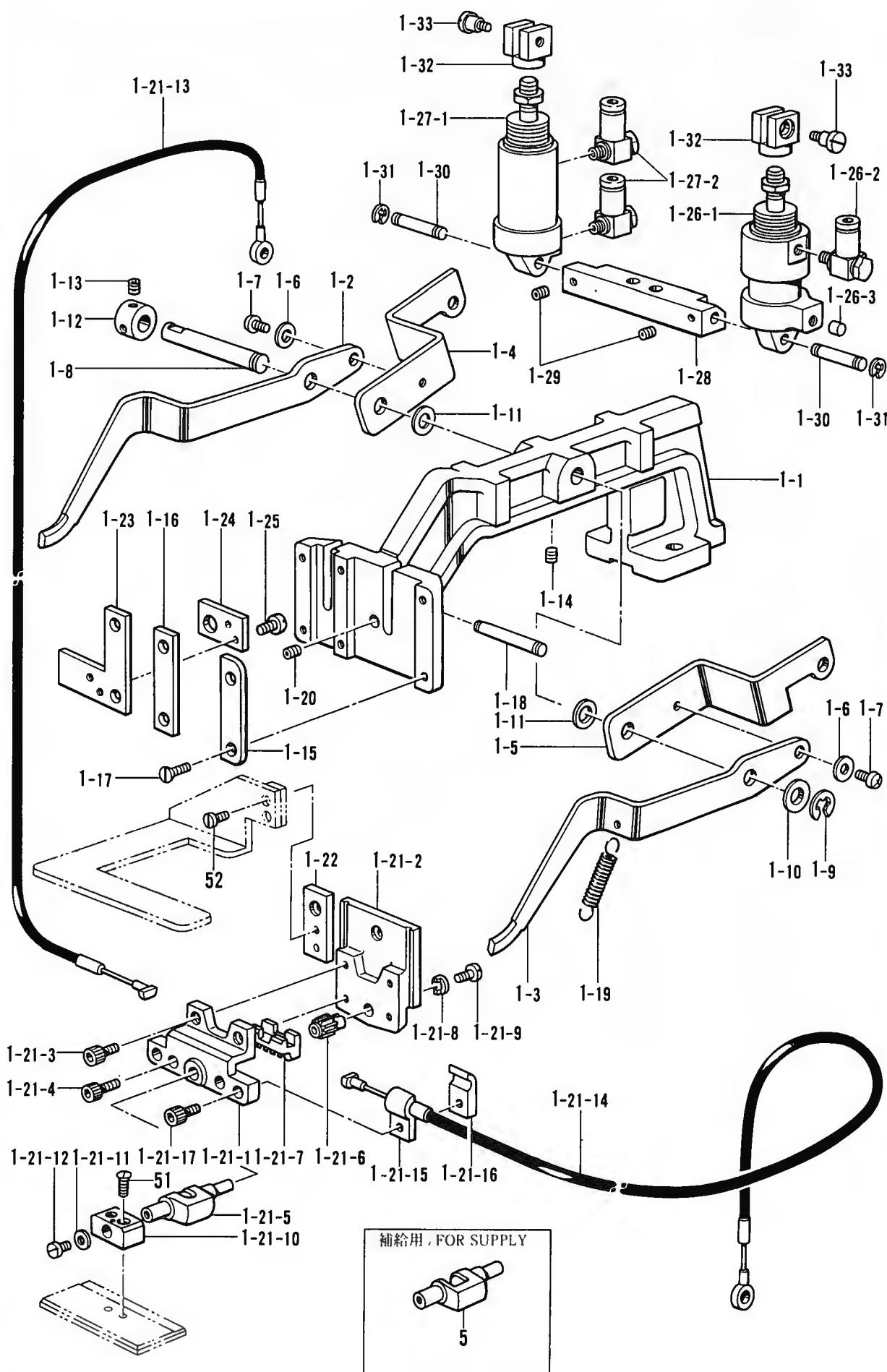
C. 送り関係/Feed mechanism/Transportvorrichtung/
