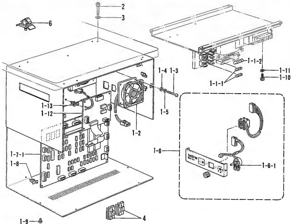
S. 電装品関係(2) / Power supply equipment mechanism (2) / Stromversorgung (2) /
