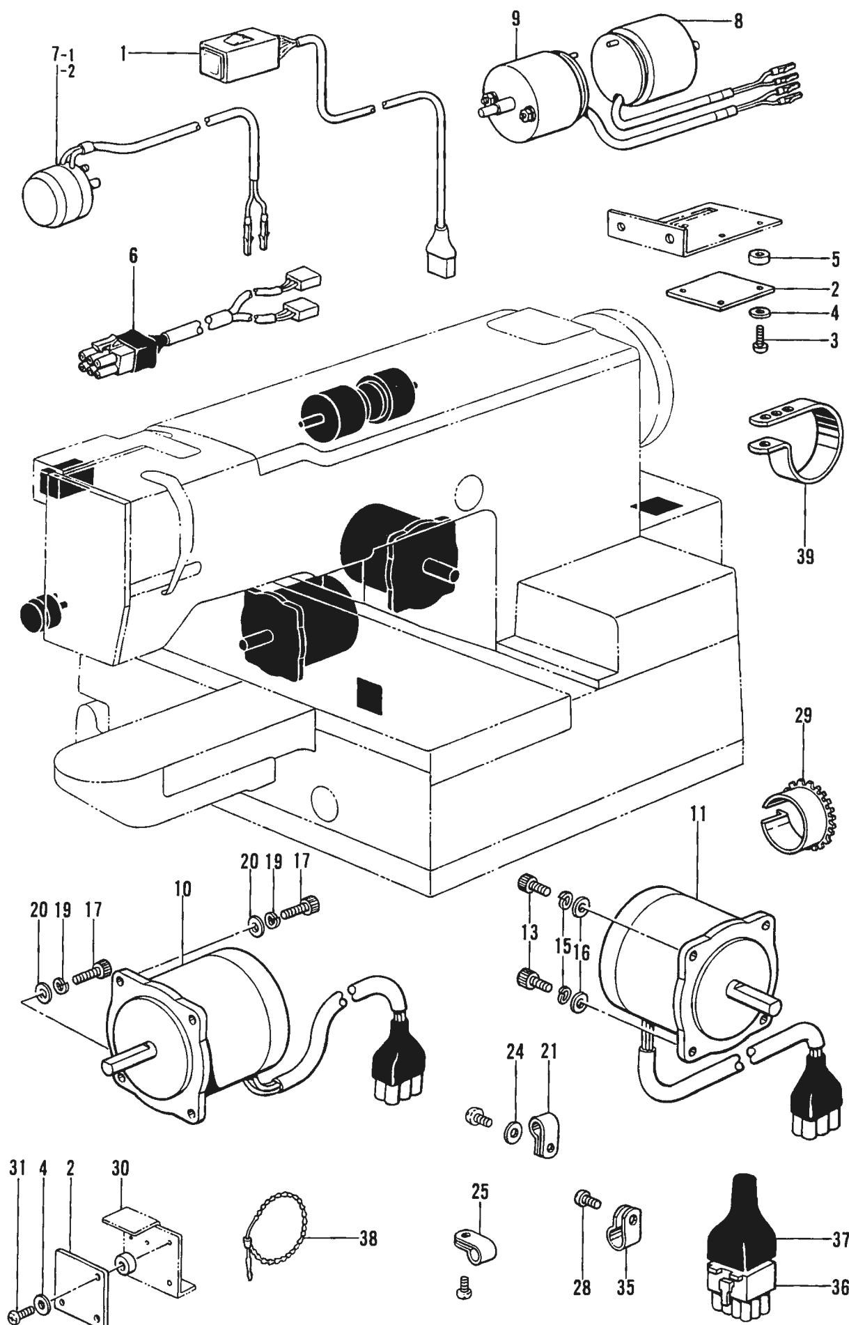
P. 電装品関係(1) / Power supply equipment mechanism (1) / Stromversorgung (1) /
